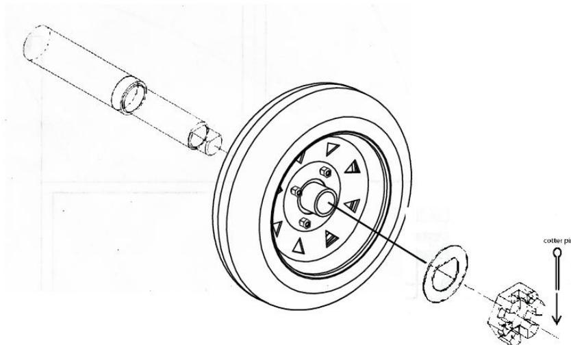
*Note: Grease the wheel bearings a minimum of 1x per year for normal use, and up to 3x per year for frequent use in order to ensure the longevity of the bearings. Adjust and re-grease the bearings after the first 100 miles.*
