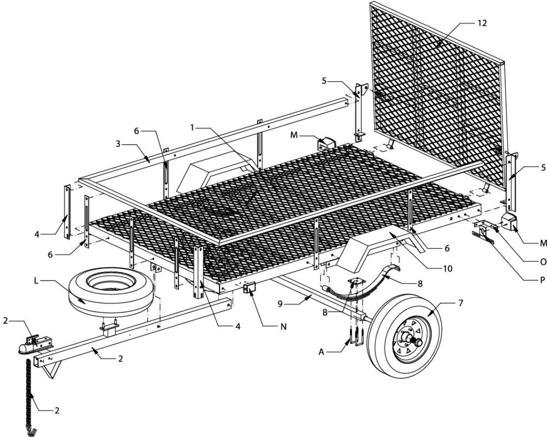
\*\*\*Spare tire mount may be located on the bottom side of the tongue so that accessories such as a gas can rack may be added.\*\*\*
